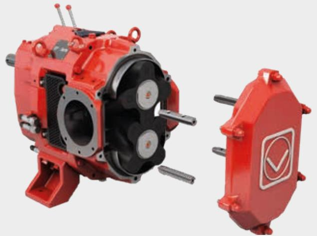
The plating concept is based on a smart fastening system consisting of four modules that are bolted from the outside. In this way, the radial wear plates are optimally positioned and can be changed very easily in the event of maintenance.
