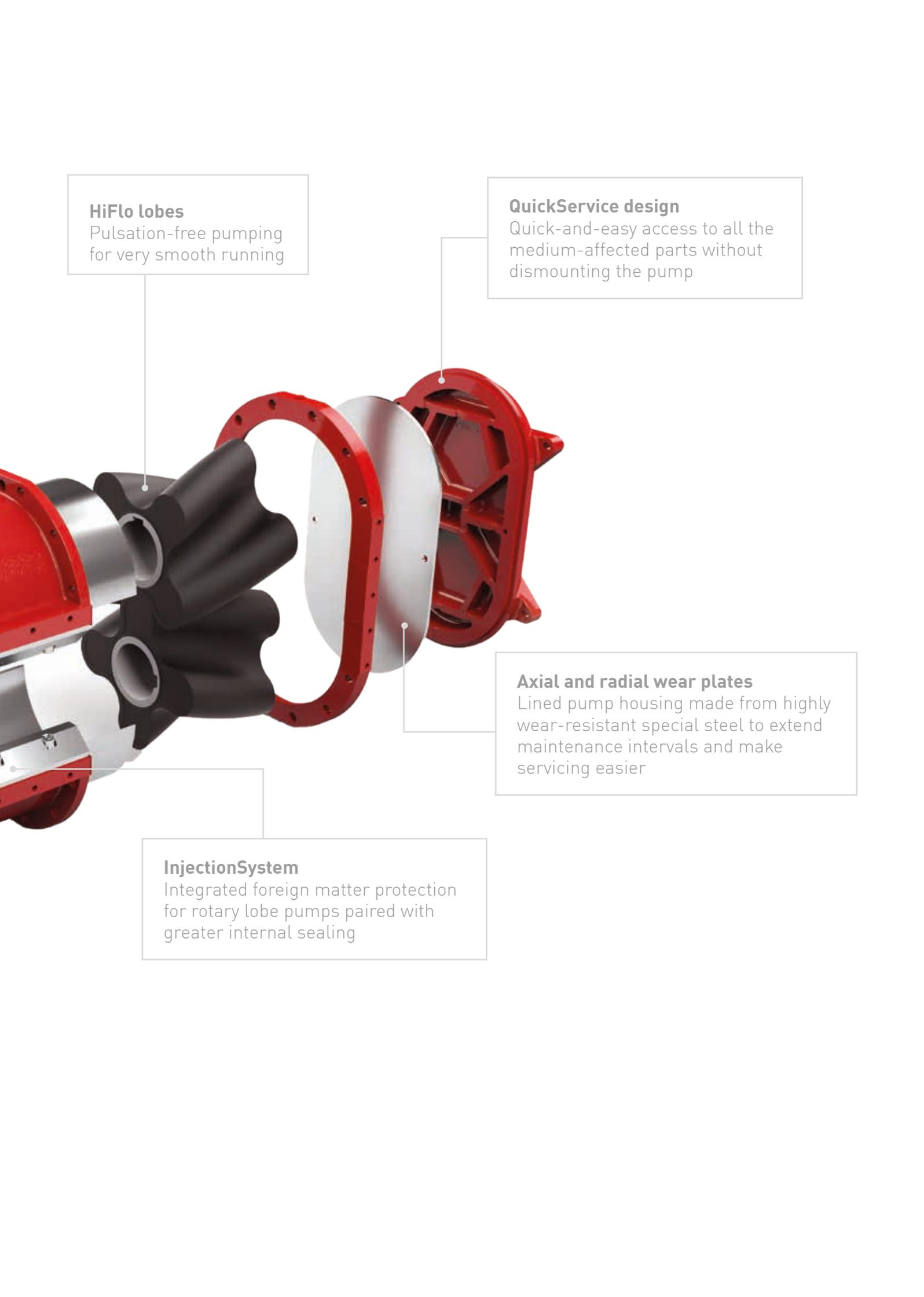
An exploded view of a rotary lobe pump assembly. The assembly consists of several main components: a red cast-iron pump housing, a silver-colored metal cover plate, a black rotor with three lobes, and a silver-colored metal injection system. The rotor is shown in the center, with the housing to its right and the injection system to its left. The cover plate is positioned between the rotor and the housing. The callout boxes are connected to the components by thin lines.
