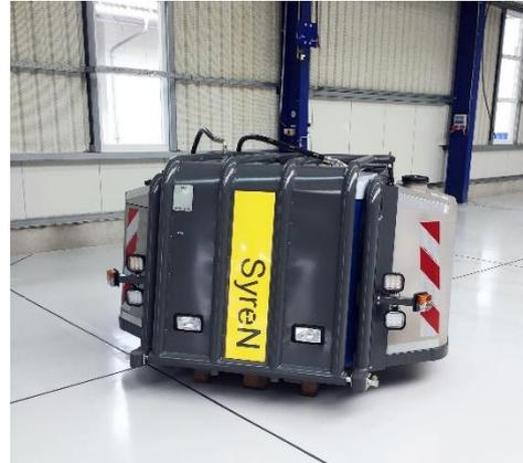
**Image 2:** The SyreN system stabilises the liquid manure by adding sulphuric acid.
