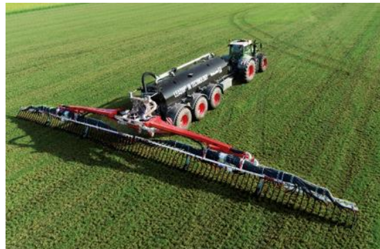
Image 4: The BlackBird trailing shoe system with a working width of 24 meters distributes the liquid manure precisely at the plant.
