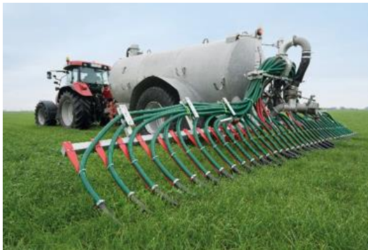
Image 3: The compact UniSpread linkage can be combined with various liquid manure outlets (here: trailing shoe).
