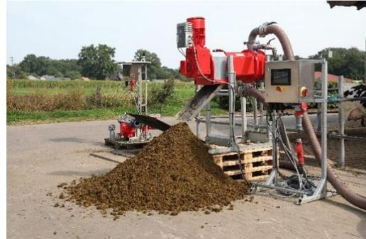
**Image 2:** The new XSplit press screw separator achieves dry matter content of up to 40 percent.
