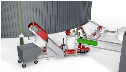
Image 1: Debris Lift Unit (DLU): fully automatic heavy material disposal during operation.
