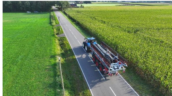
Image 4: With an arm length of 9 meters in transport position (measured from the lower link), the new large BlackBird can be attached to a wide range of liquid manure tankers.
