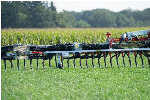
Image 3: Four ExaCut ECM precision distributors are installed as standard in the new 30-meter trailing shoe linkage.
