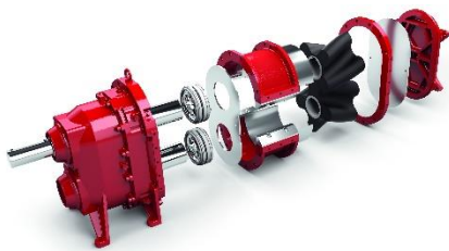
Image 3: The exploded view of a VX series rotary lobe pump.
