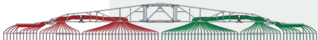
Half-boom section switch-off
