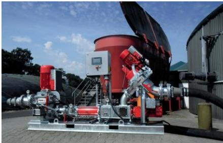
**Image 2:** In use: compact unit for mechanical disintegration consisting of RotaCut, CC series progressive cavity pump, DisRuptor and a PCU controller.
